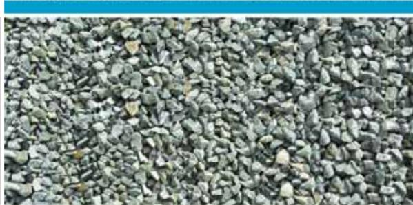
4 inch well compacted, large, single size, crushed stone which meets DOT specifications for a porous application
