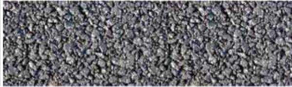
2 inch open-graded porous bituminous base course which meets DOT specifications for a porous application
